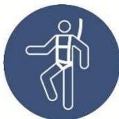
A fall protection personal protection equipment equipped with an energy absorber has to be used when using the system (corresponding to PSAgA EN 361 and EN 363), and the acting forces must be reduced to less than 6 kN. The stipulations issued by the manufacturer of the equipment used must be observed.
