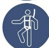
A fall protection personal protection equipment equipped with an energy absorber has to be used when using the system (corresponding to PSSaG A EN 361 and EN 363), and the acting forces must be reduced to less than 6 kN. The stipulations issued by the manufacturer of the equipment used must be observed.
